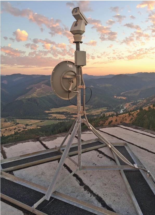
An Oregon Department of Forestry wildfire detection camera monitors thousands of acres of forestland, using artificial intelligence and mapping technology to detect smoke and help dispatch firefighters quickly.
