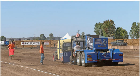
The Iron Mule sled follows an amateur competitor down the dirt track. As the sled moves forward, increasing resistance makes it progressively harder for the truck to continue its pull.
